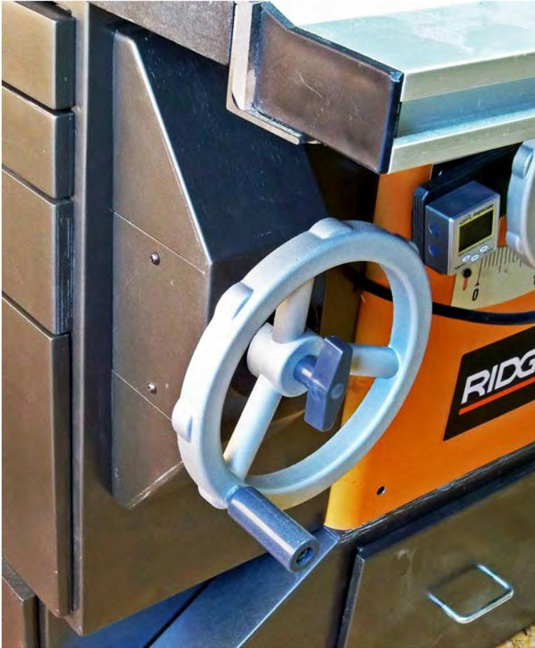
*Front-Mounted Tilt Handwheel*
